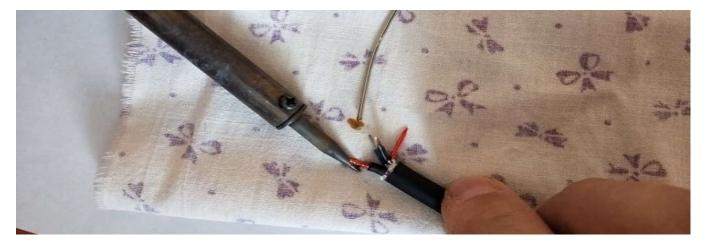
You should also 'tin' both contacts before you attempt to solder them. This will coat the wires or connector contacts with solder so you can easily melt them together. Make sure there are no loose stands of wire during this process.
