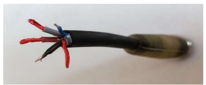
You'll see in this photo the red varnish on the wires once they're stripped back ready for soldering, it's essential this varnish is burnt off the wires prior to tinning so ensure good solder adhesion. Use the soldering iron tip to burn the varnish off the red coloured wires. It is essential all varnish is removed prior to soldering to prevent solder adhesion failure.
