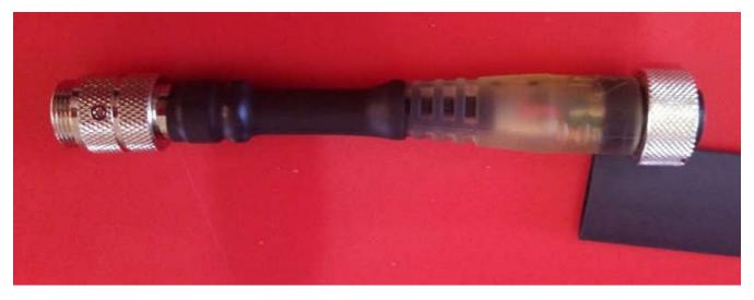
The last step we take to add strength is to wrap the entire adapter in a tough tape, you can use any tape you prefer, electrical tape is an easy choice. There are plenty of good quality strong adhesive tapes you could use for the task, the other option is some large dual wall heat shrink that fits over the plugs to shrink down onto the adapter.
