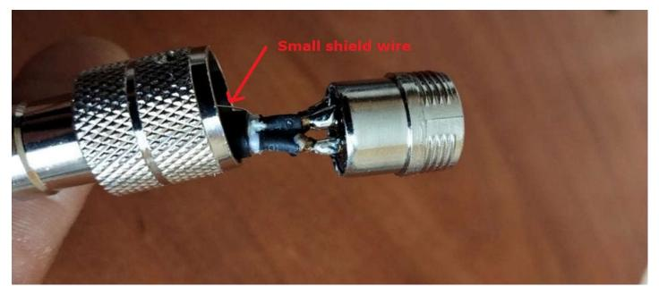
You should now be able to check all the wires to ensure no stray wire is touching any other wire or pins causing any shorts, this is very important. Your solder should be smooth and shiny, not rough. The image below demonstrates what a good solder connection should look like.
