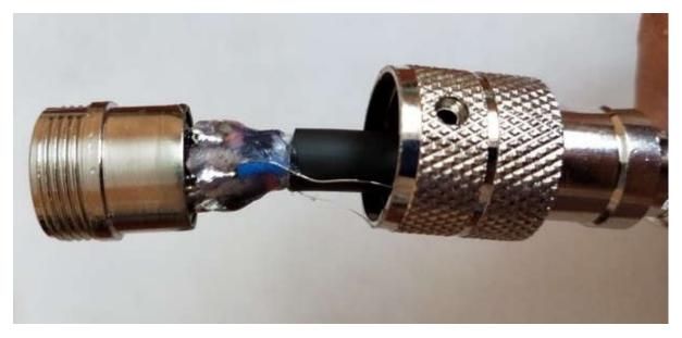
In the above photo the hot glue has been applied, all pins and wires were checked for shorting and the ground wire is coming off the blue wire out to the back of the microphone plug. We now need to shrink the heat shrink we've got waiting on the cable over the top of the hot glue.
