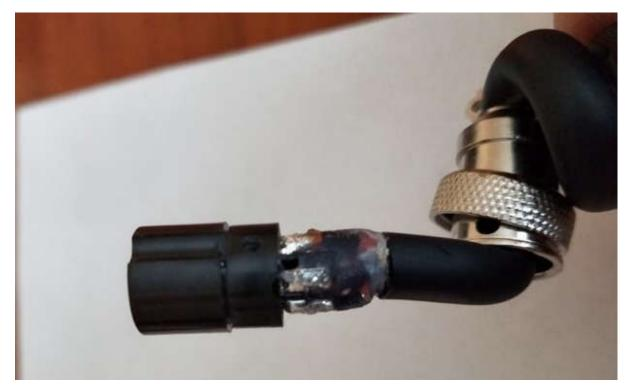
You can now use your original Z-7K coil which you cut the end off by using the adapter for your X-coils. If you have another size OEM Z-7K coil without the end removed, you'll be able to use it as per normal without the adapter.
